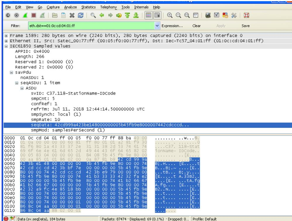
Figure 2-3 Captured synchrophasor multicast sampled values frame
