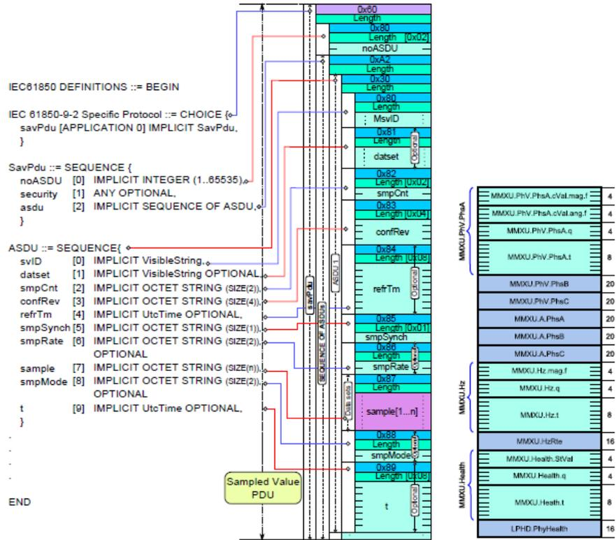
Figure 2-2 Encoding of the SV APDU frame and synchrophasor data (at right)
