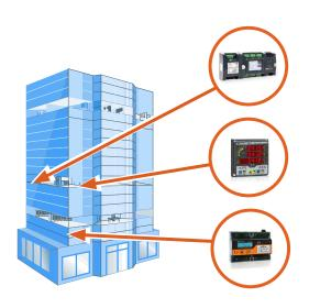
**Preventing utility errors:** metering electricity independently of the utility provider, along with generating an energy balance within the site, allows facility managers to easily detect utility errors and prevent overcharges.
