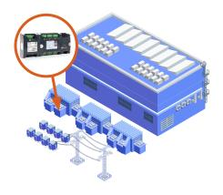
Typically, industrial plants have many loads that are fed from the same MCC. It has been proven that online monitoring of the consumption down to a single load level results in energy saving of up to 30%. Utilizing the BFM-II is the most compact and efficient method for monitoring several loads located up to 200m from
