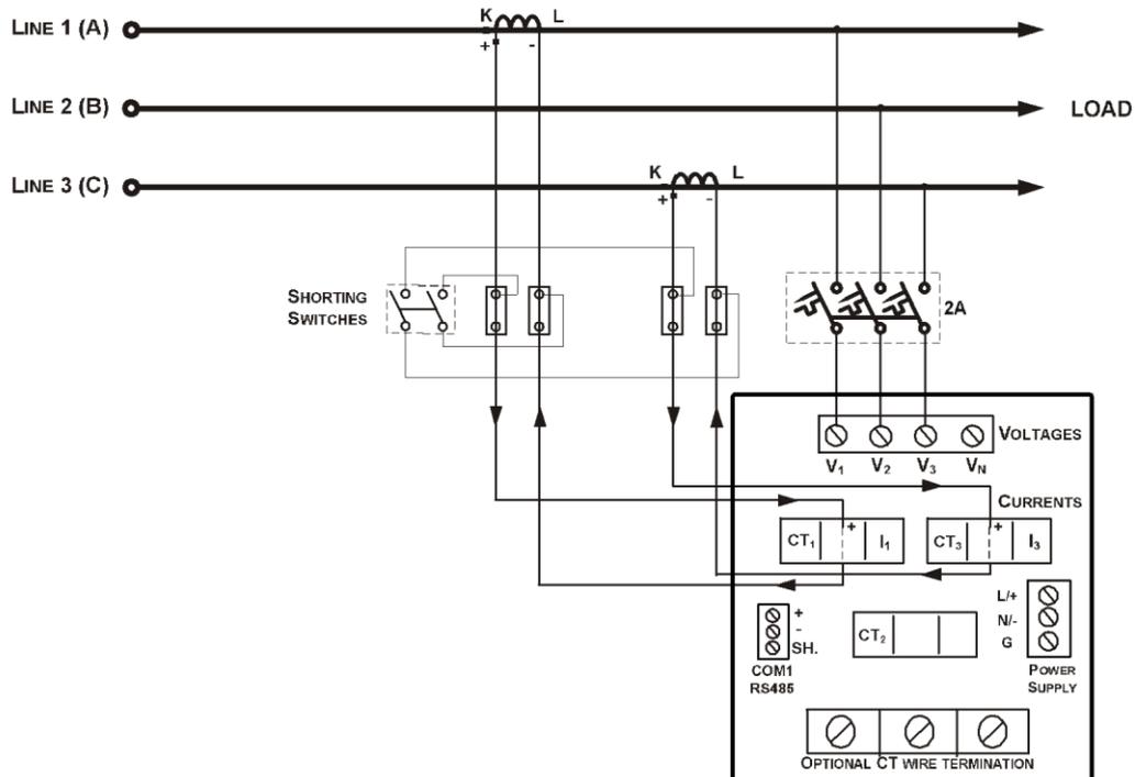
**Figure 2-9 3-Wire 2-Element Delta Direct Connection Using 2 CTs (Wiring Mode = 3dir2)**
