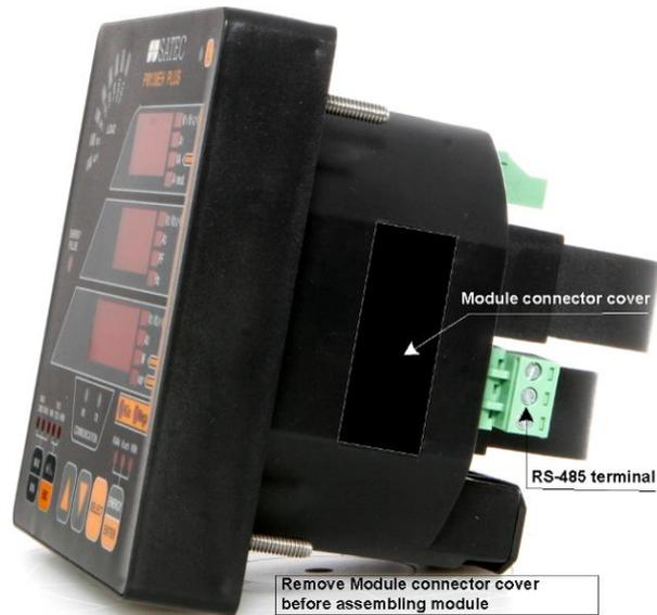
**Figure 2-21 Module Connector Cover – Before Module Assembly**
