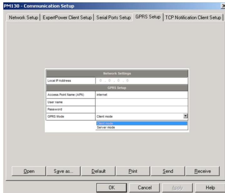
Figure 5-3: Communication Setup Dialog Box – GPRS Setup Tab
