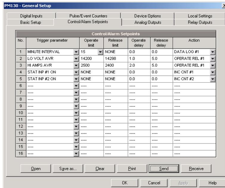
**Figure 5-12: General Setup Dialog Box – Control/Alarm Setpoints Tab**
