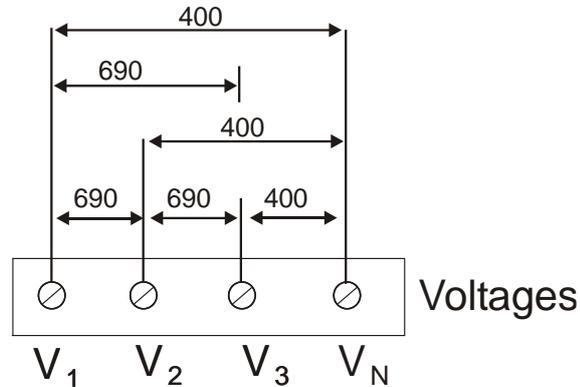
690V inputs are usually used with direct connection. Use any of the seven wiring configurations shown in Figures 2-8 through 2-15.
