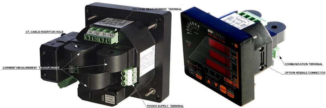
Figure 2-7 Terminals - Rear View
