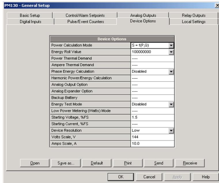
Figure 5-7: General Setup Dialog Box – Device Options Tab
