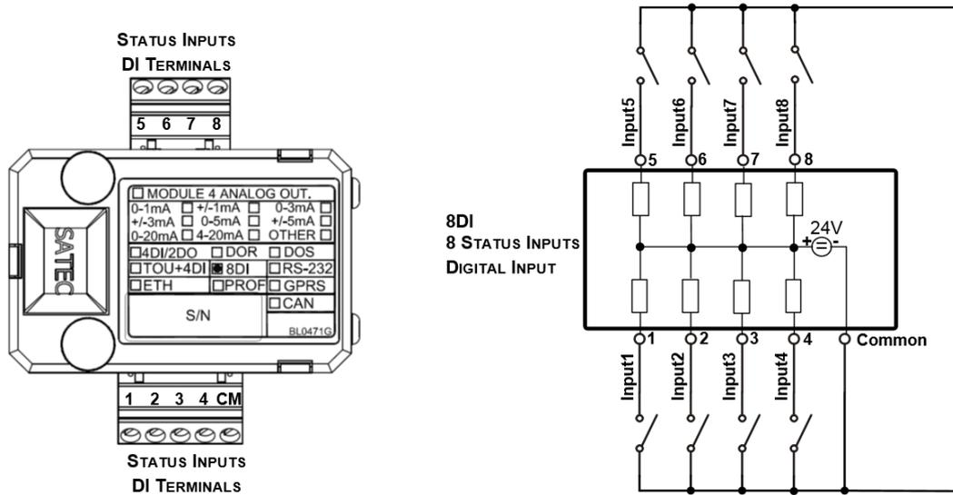
Figure 2-25 8 DI - Digital Input Connection
