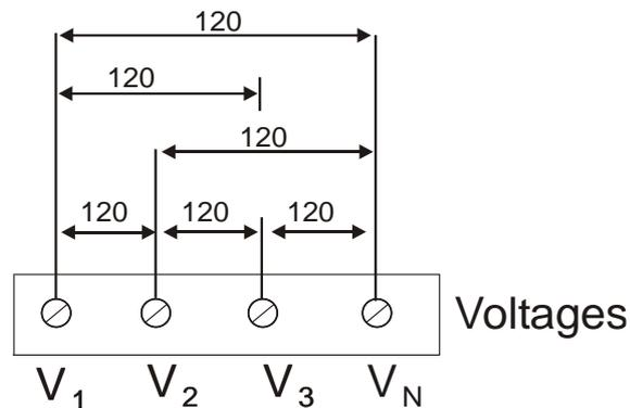
120V inputs usually imply use of a potential transformer (PT). The PT requires use of any of the four wiring configurations shown in Figures 2-7 through 2-10.
