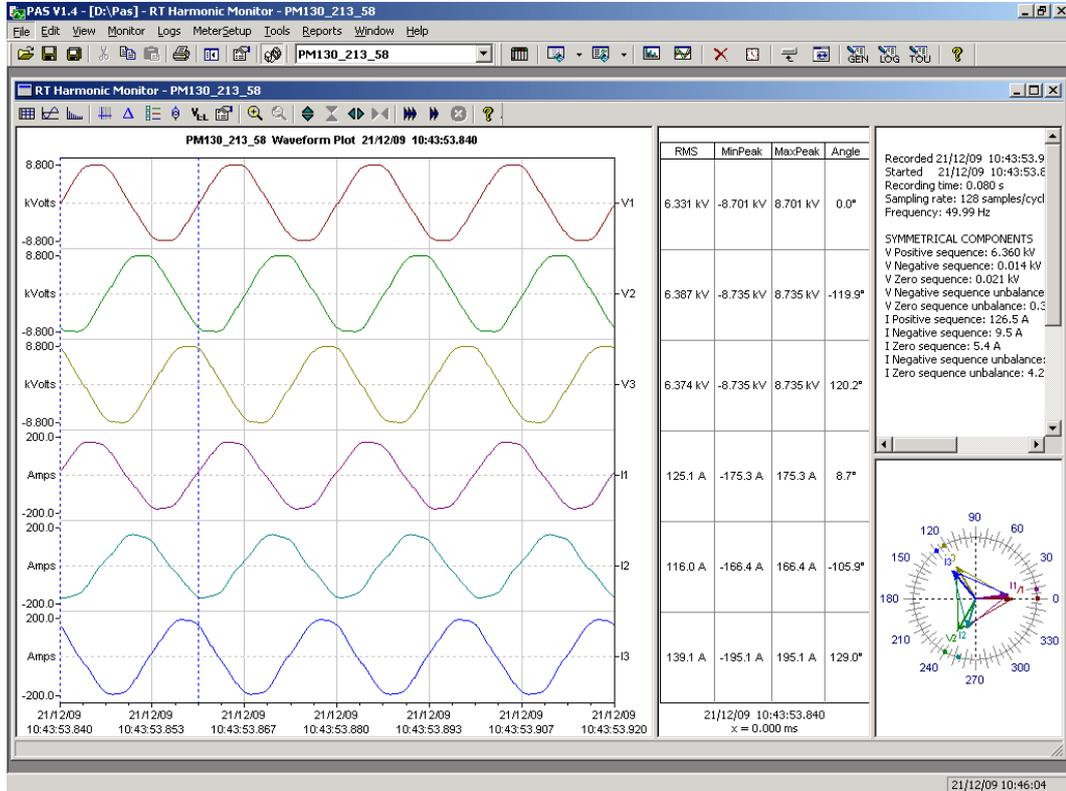
Figure 7-6: RT Harmonic Monitor – Synthesized Waveforms
