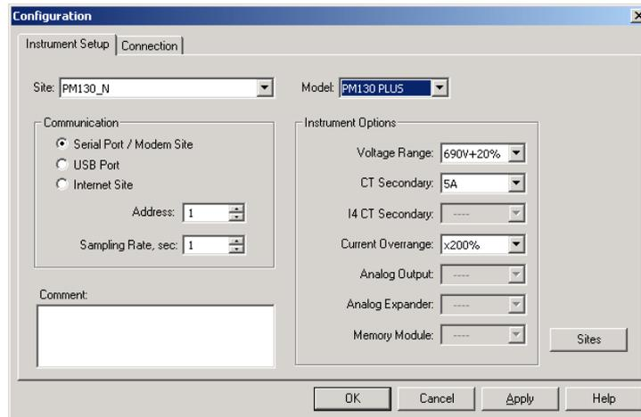
Figure 4-1: Configuration Dialog Box – Instrument Setup Tab
