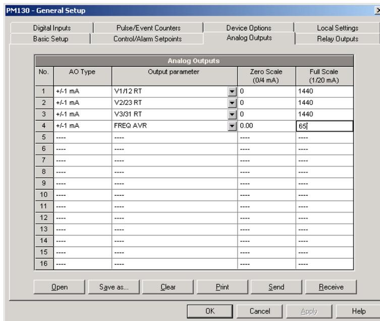
Figure 5-10: General Setup Dialog Box – Analog Outputs Tab
