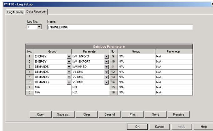
Figure 5-19: Log Setup Dialog Box – Data Recorder Tab
