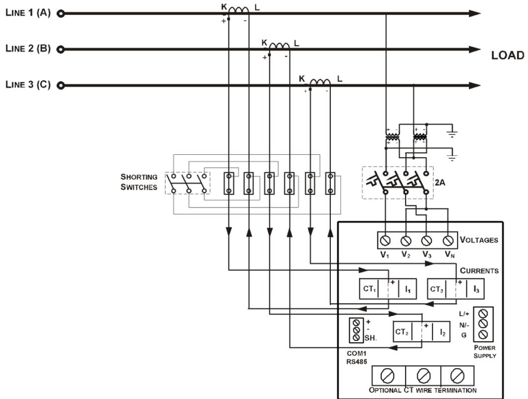
Figure 2-16 3-Wire 2½-Element Broken Delta Connection Using 2 PTs, 3 CTs (Wiring Mode = 3bLn3 or 3bLL3)
