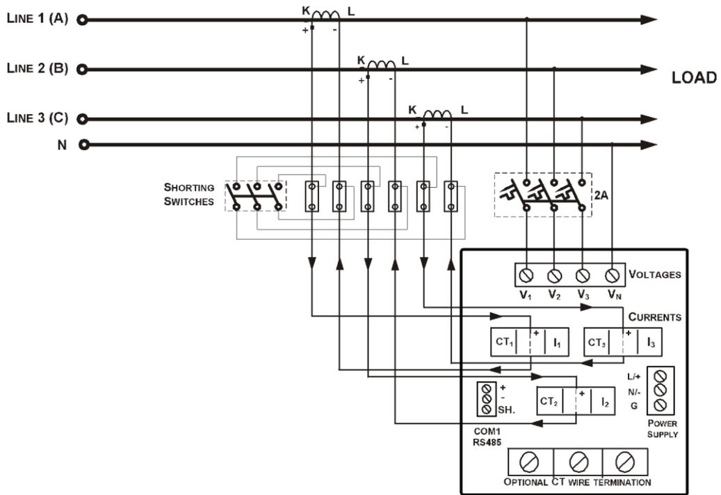
Figure 2-10 4-Wire Wye 3-Element Direct Connection Using 3 CTs (Wiring Mode = 4LL3 or 4Ln3)
