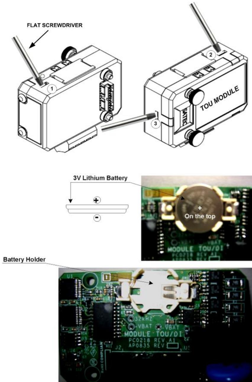
Figure 2-31 TOU RTC Battery Replacement
