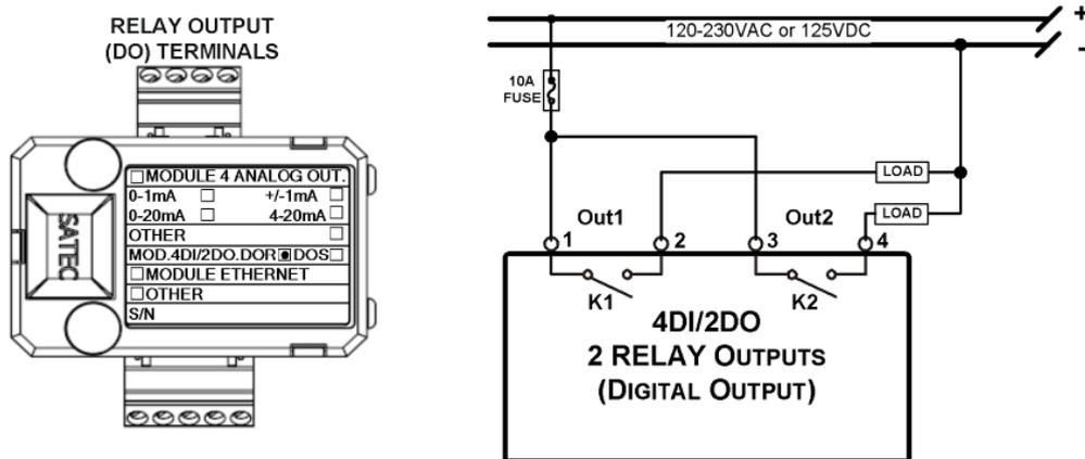
Figure 2-23 Relay Output Connection
