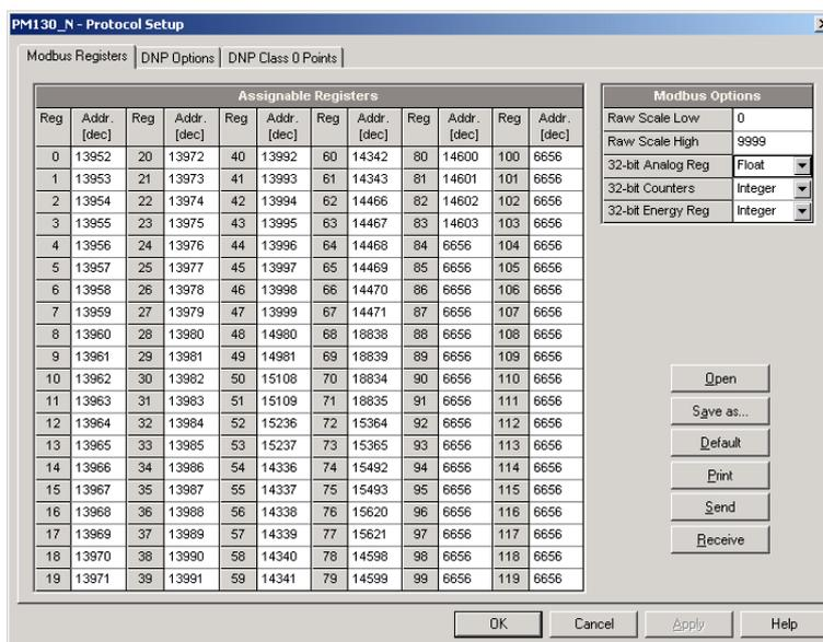
Figure 5-20: Protocol Setup Dialog Box – Modbus Registers Tab
