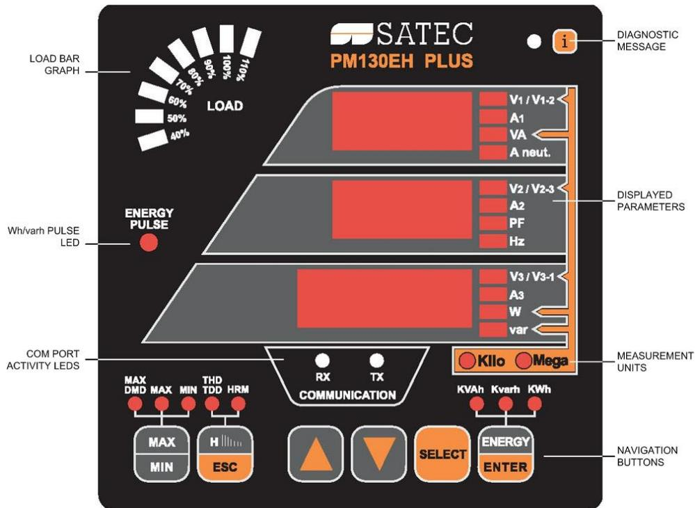
Figure 3-1: PM130 PLUS Unit (AC Current mode)
