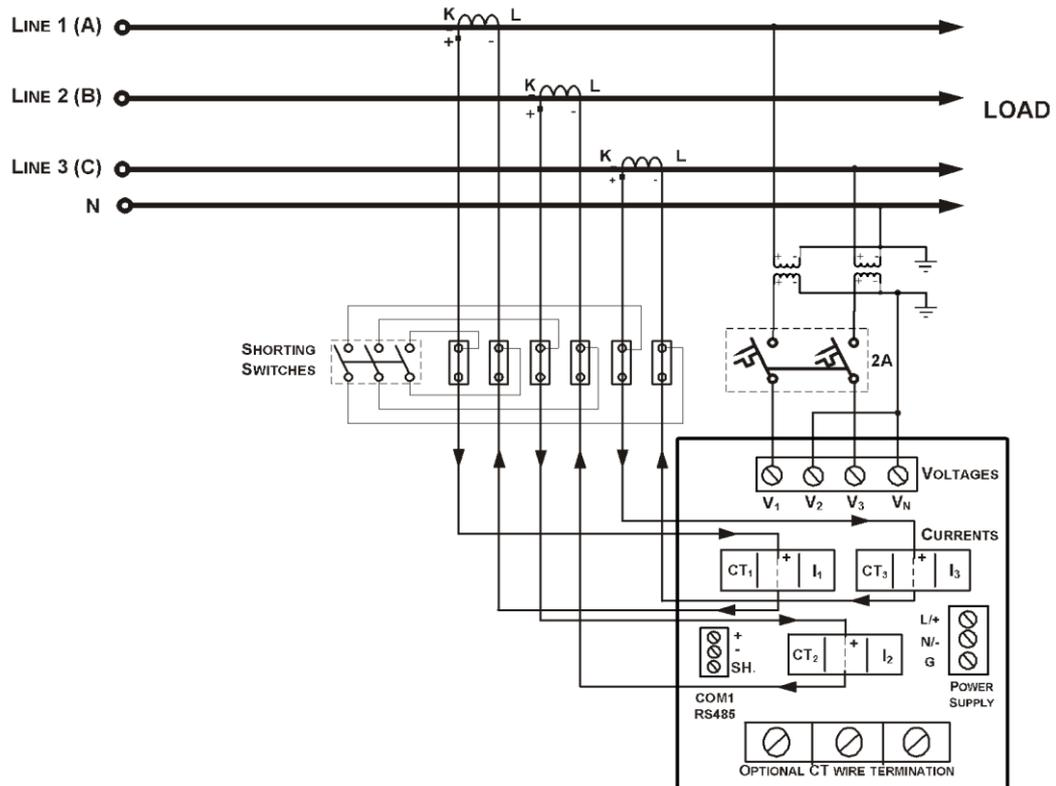
This configuration provides accurate power measurements only if the voltages are balanced.
