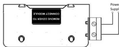
Figure 2-9 Auxiliary Power Supply Connection
